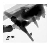
ZnO prepared by chemical vapour deposition with gold loaded by ultrasonication was very active for CO oxidation. The unique catalyst–substrate interaction (epitaxy related) might be related with the results observed.
