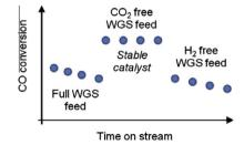
The predominant active state in Au/CeZrO<sub>4</sub> catalysts for low-temperature water gas shift is thought to be Au(0) and, through varying the reaction feed conditions, it was possible to enhance the stability of the catalysts significantly.
