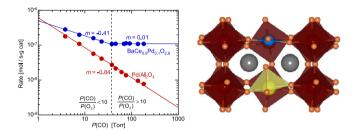
Low surface area, crystalline  $Ba(Ce,Pd)O_3$  catalyzes CO oxidation using either oxygen adsorbed from the gas phase or labile lattice oxygen, and the rate law depends strongly on the  $P(CO)/P(O_2)$  ratio. Catalytic activity is attributed to the presence of square-planar Pd(II) ions located on the perovskite B-sites, each adjacent to an oxygen vacancy.
