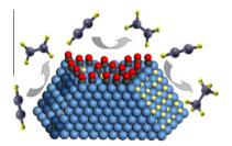
The selectivity of alkyne hydrogenation on Pd depends on the subsurface chemistry. CO blocks the dynamic state of the catalyst and turn it into a robust, selective configuration.
