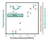
The relationship between the nature of W surface species, acidity and activity, was established for a series of  $WO_x/Al_2O_3$  catalysts. Polymeric W surface species were found to be directly related to the abundance of relatively strong Brønsted acid sites and to the development of the catalytic activity for isopropanol dehydration.
