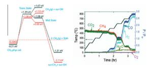
Energy level diagram (calculated) for breaking the C–H bond of methane. Steady state output from the reactor at different temperatures, for methane dry reforming. The catalyst is Pt-doped CeO<sub>2</sub>.
