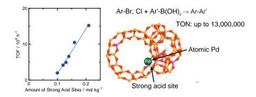
Pd loaded on USY zeolite exhibited very high activity in Suzuki-Miyaura reactions. The active species was proposed to be the atomic Pd anchored to the strong acid sites of USY.
