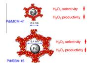
SBA-15 allows preparing palladium catalysts with enhanced productivity and selectivity in the direct synthesis of hydrogen peroxide by imparting Pd particles the proper size and distribution.
