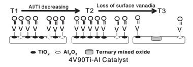
Surface active vanadia species present on  $TiO_2$ - $Al_2O_3$  mixed oxide support depends on loading and calcination temperature. Surface Al/Ti ratio varies with calcination temperature and depends on vanadia loading.
